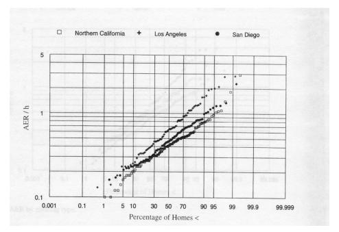
Figure 2. Air exchange rate by study area measured during the winter of 1991-1992.
