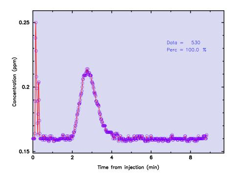
Figure 17. Decimal time-concentration data file for the Tracq04.prn data file developed from a short-term column study (100% of the data shown).
