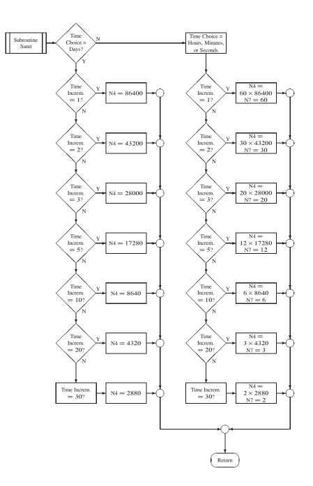
Figure 10. Flowchart depicting subroutine for memory size determination based on seconds.
