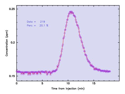
Figure 16. Decimal time-concentration data file for the Tracq01.prn data file developed from a short-term column study (20.1% of the data shown).
