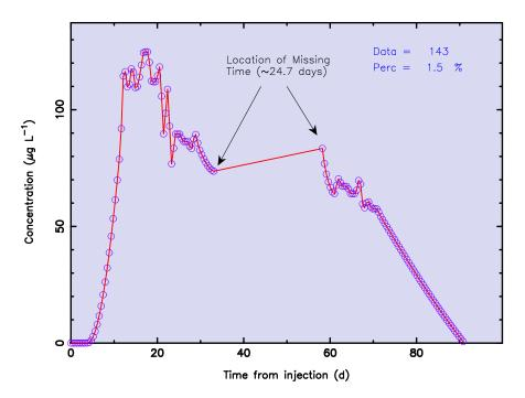
Figure 48. Decimal time-concentration data file for the Break.prn data file developed from a 5 km tracer test (1.5% of the total data shown). Note arrows indicating the location of missing time.
