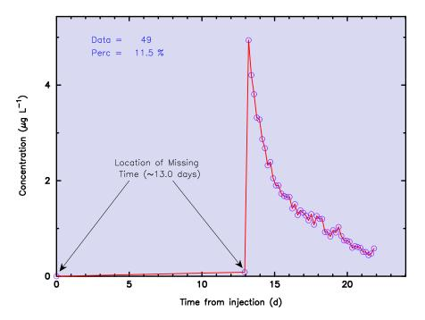
Figure 51. Decimal time-concentration data file for the 03g158.prn data file developed from a tracer test ( $\sim$ 11% of the data shown). Note arrows indicating the location of missing time.
