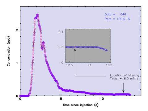
Figure 39. Decimal time-concentration data file for the Creek.prn data file developed from a 2 km tracer test (100% of the data shown). Note arrow indicating the location of missing time.
