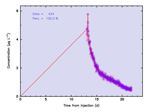
Figure 52. Decimal time-concentration data file for the 03g158.prn data file in which the second (12.9434,0.086) and last (21.8634,0.123) data points have been deleted using FLOWTHRU.
