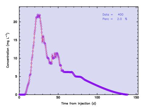
Figure 46. Decimal time-concentration data file for the Fluor\_time.prn data file developed from a 5 km tracer test and set for 2% of the data as shown.
