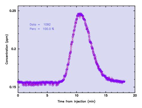
Figure 15. Decimal time-concentration data file for the Tracq01.prn data file developed from a short-term column study (100% of the data shown).
