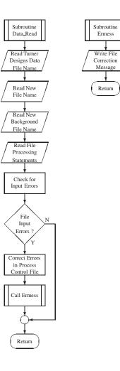
Figure 8. Flowchart depicting subroutine for implementing interprocess control file and error reporting.
