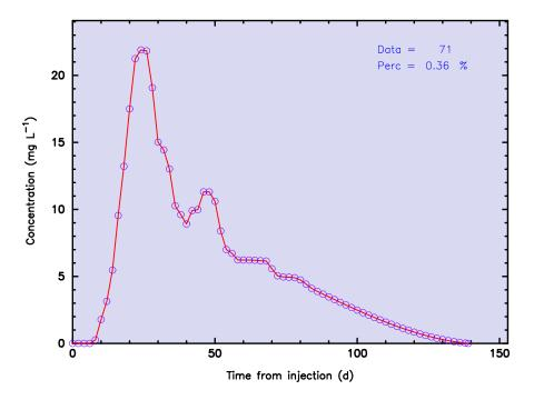
Figure 43. Decimal time-concentration data file for the Fluor\_time.prn data file developed from a 5 km tracer test where data are processed for every other day (0.36% of the data shown).
