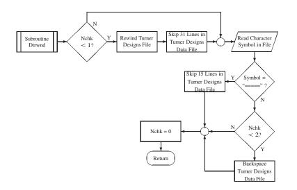
Figure 11. Flowchart depicting subroutine for counting past Turner Designs header and separate data blocks.
