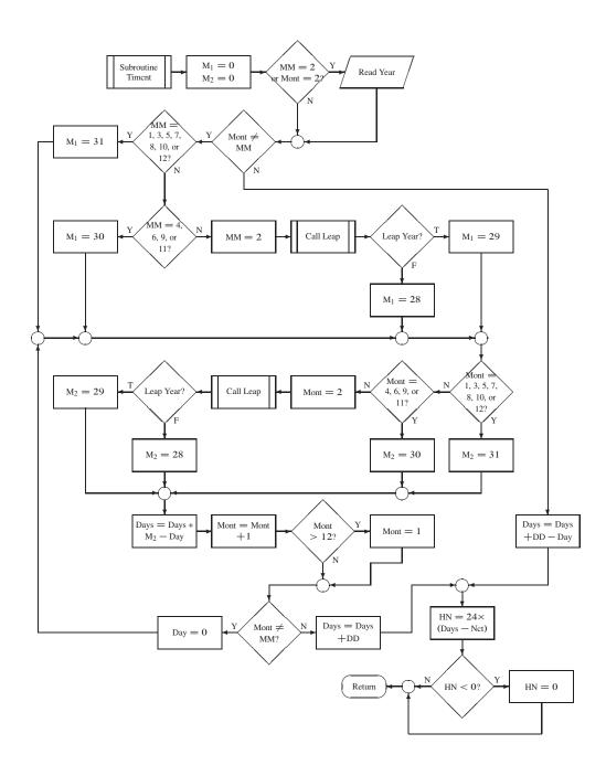
Figure 12. Flowchart depicting subroutine for counting past time breaks in the Turner Designs data file.
