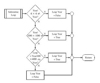
Figure 13. Flowchart depicting subroutine for determining whether time breaks in the data occurred in February during a leap year.
