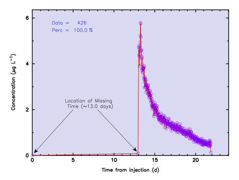
Figure 49. Decimal time-concentration data file for the 03g158.prn data file developed from a tracer test (100% of the data shown). Note arrows indicating the location of missing time.
