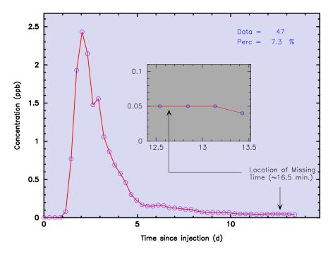
Figure 40. Decimal time-concentration data file for the Creek.prn data file developed from a 2 km tracer test (<10% of the data shown). Note arrow indicating the location of missing time. Also note expanded graph inset with missing time more prominently depicted.
