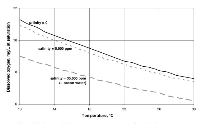
Figure 10. Oxygen solubility versus temperature at various salinities.
