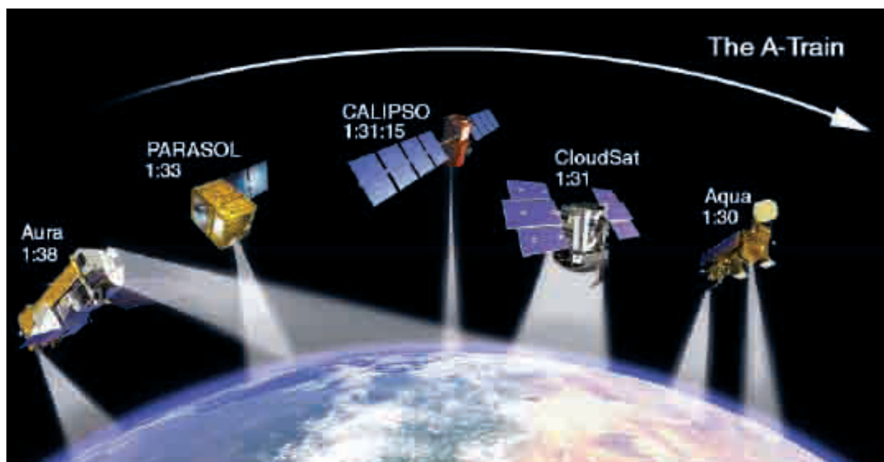
Figure 9-60. A constellation of five spacecraft that overfly the Equator at about 1:30 PM, the so-called A-Train, carries sensors having complementary capabilities, offering unprecedented opportunities to study aerosols from space in multiple dimensions.
