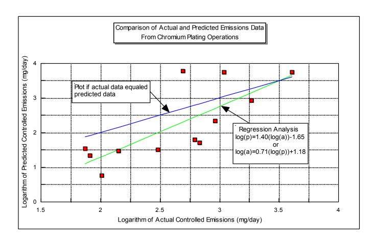
*Figure 1.* Comparison of Actual and Predicted Emissions Data from Chromium Plating Operations.
