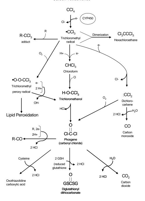
Figure 3-1. Metabolic scheme for carbon tetrachloride.
