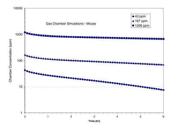
Data points are observations (provided by Thrall) for exposures for seven mice per chamber (body weight, 0.024 kg); lines are simulations. The non-specific loss rate of CCl<sub>4</sub> from the chamber was assumed to be 0.05 hour<sup>-1</sup> (from Thrall source code). Partition coefficients were from Thrall source code.
