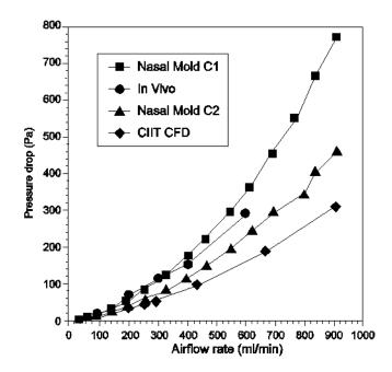
Figure 3-11. Pressure drop vs. volumetric airflow rate predicted by the CIIT
