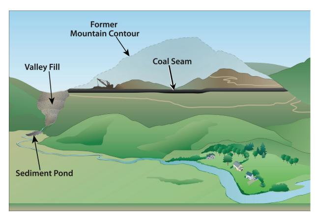
Figure 4. A watershed view of a mountaintop mine and valley fill (no consistent scale).
