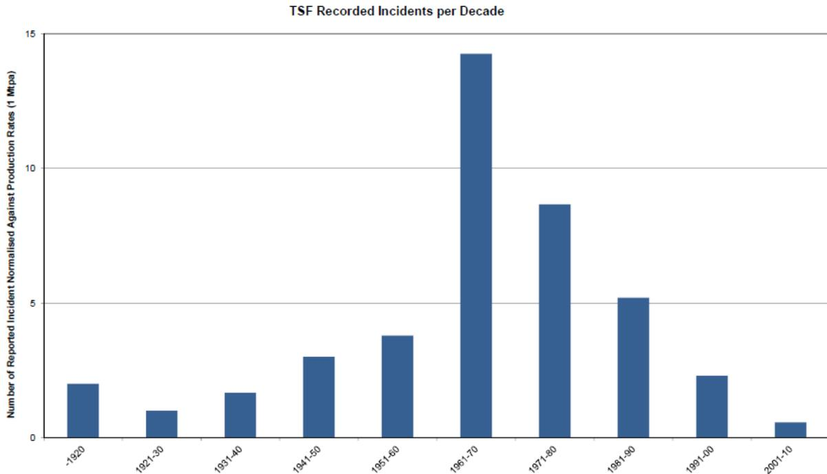
**Figure 2. TSF Failures/Mtpa tailings production<sup>2</sup>**
