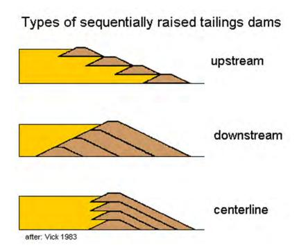
Downstream construction is the safest type of construction from a seismic standpoint, but is also the most expensive option.
