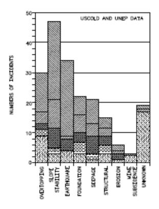
Figure 9. Tailings dam incident cause comparison with dam type.
