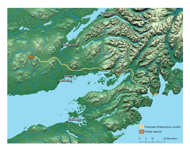
**Figure 2**. Anticipated location of the road, pipeline, and utility transmission corridor for Pebble Mine (Ghaffari et al. 2011, p. 326). The new road and pipeline corridor would connect the Pebble Mine operations with a new seaport on Cook Inlet. Not shown is an existing north-south connecting tie road from near Nondalton to the Iliamna area (see Figure 1). The Pebble segment from Cook Inlet west to near Lake Iliamna would be reconstructed over an existing lower-standard roadway.
