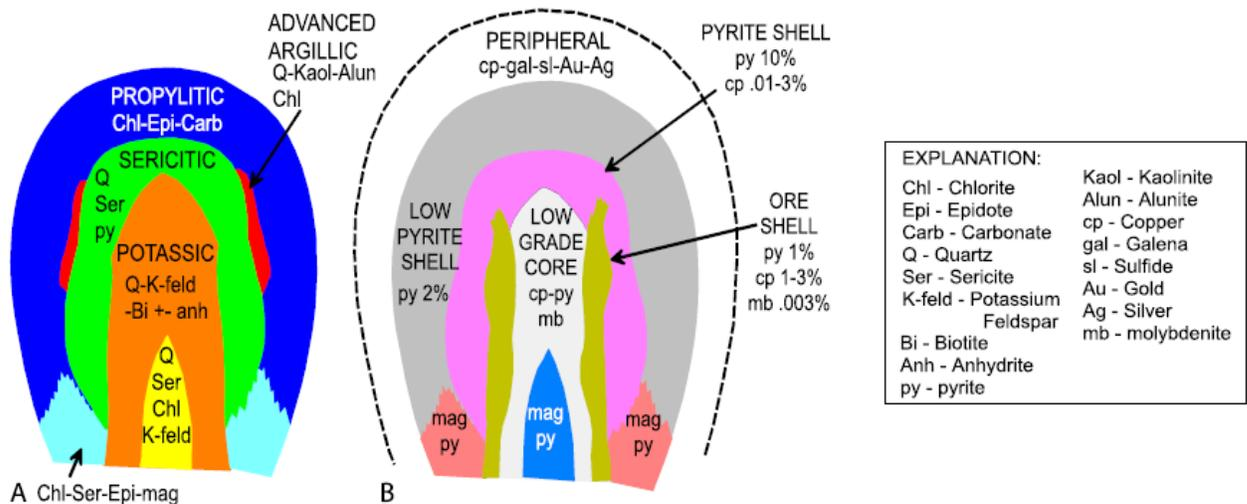
**Figure 3.** Idealized cross section through a porphyry copper deposit showing the relationship of the ore zone to various alteration types. A. Distribution of alteration types; B. Distribution of ore mineral assemblages. The causative intrusion corresponds to the potassic alteration zone. From John and others (2010) and modified from Lowell and Guilbert (1970).
