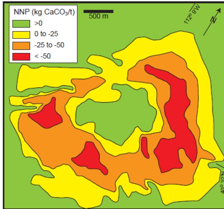
**Figure 6.** Plan view of the distribution of net neutralizing potential (NNP) values at the Bingham Canyon porphyry copper deposit, Utah. NNP values above zero are “net alkaline”; those below zero are “net acid”. Modified from Borden (2003).
