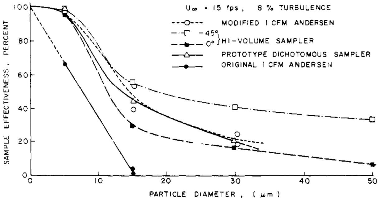
Different TSP sampler types: (1) Modified Andersen Sampler [open circles]; (2) Hi-volume Sampler (for different incident wind direction (45° [open squares], 0° [closed squares])); (3) Prototype 15  $\mu\text{m}$  Cutpoint Dichotomous Sampler [open triangles]; and (4) Original Andersen Sampler [closed circles].
