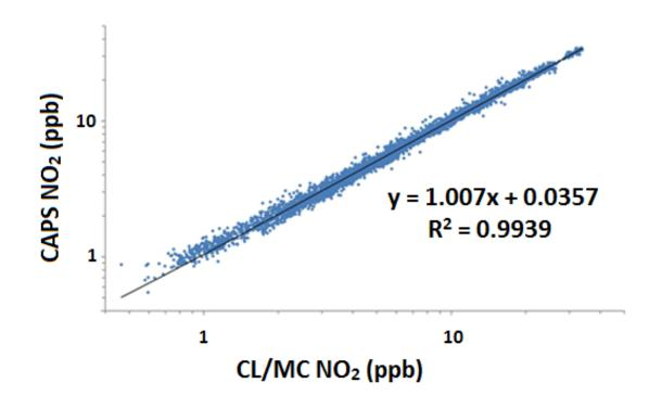
Note: CAPS = cavity attenuated phase shift, CL/MC = chemiluminescence/MoO<sub>X</sub> catalytic converter, NO<sub>2</sub> = nitrogen dioxide. Source: National Center for Environmental Assessment 2013 analysis of data from <u>Kebabian et al. (2008)</u>.
