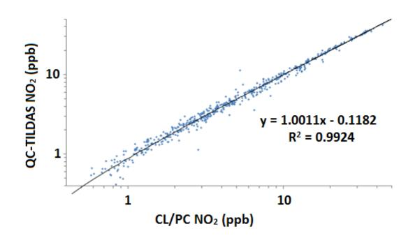
Note:  $NO_2$  = nitrogen dioxide, PC = photolytic converter, QC-TILDAS = quantum cascade-tunable infrared differential absorption spectroscopy.
