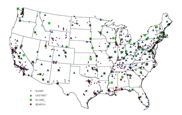
Note: SLAMS = State and Local Air Monitoring Stations, CASTNET = Clean Air Status and Trends Network, NCORE = National Core Network, SEARCH = Southeast Aerosol Research Characterization. Source: U.S. Environmental Protection Agency 2013 analysis of data from monitoring networks.
