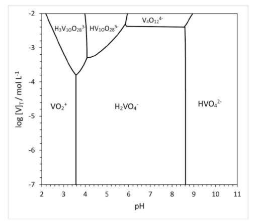
Fig. 3. Predominance diagram showing the speciation of vanadate (V) as a function of pH and total concentration of vanadium,  $[V]_T$ . T = 25 °C, I = 0.01 mol L<sup>-1</sup> (as NaCl). To produce the diagram, equilibrium constants selected for Visual MINTEQ were used (Table S3).
