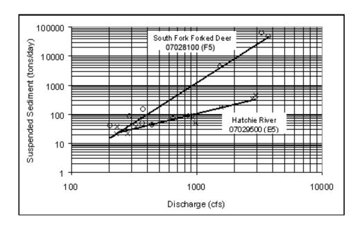
**Figure 5:** Suspended sediment transport curves for South Fork, Forked Deer and Hatchie River (from Simon, 1989).
