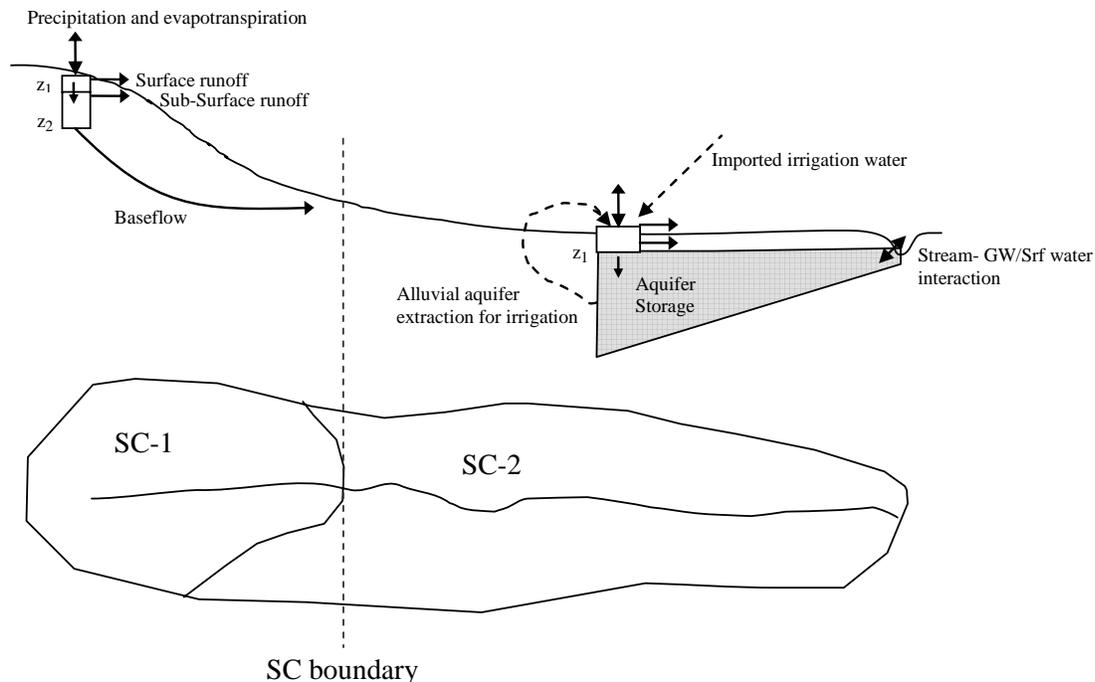
**Figure 4.3.** This schematic shows a watershed broken into two sub-catchments. SC-1 is a headwater catchment, without surface-groundwater interaction and applies the two “bucket” water balance model. SC-2 is characterized as being in a valley area, where the surface hydrology applies the single bucket water balance with recharge to an underlying alluvial aquifer which as groundwater-surface water interaction.
