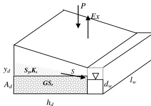
**Figure 4.5. Schematic of the stylized groundwater system, and its associated variables.**
