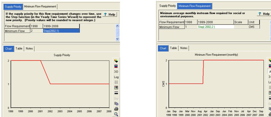
Figure 4.7. WEAP21's GUI for specifying instream flow requirements. The left panel shows the supply priority of instream flow, while the right panel is the actual instream flow requirement in  $m^3/s$  that abruptly change over time as a result of regulatory requirement.
