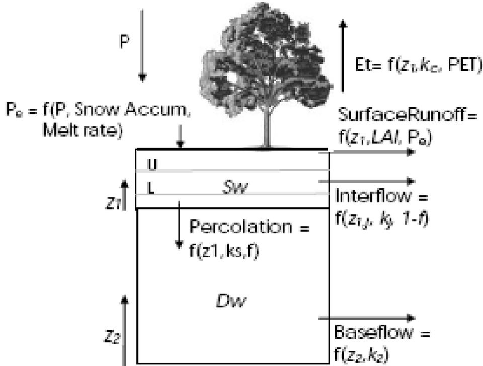
**Figure 4.4. Schematic of the two-layer soil moisture store, showing the different hydrologic inputs and outputs for a given land cover or crop type,  $j$**
