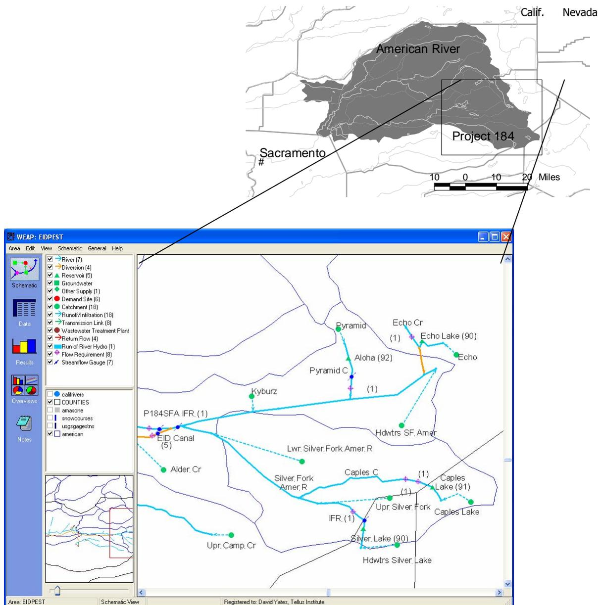
**Figure 2.** EID's Project 184 system as represented in the WEAP DSS. The 10 dots and their connecting dotted lines represent individual sub-catchments (Pyramid, Echo, Headwaters South Fork American, etc.). The four triangles are the reservoirs (Silver, Caples, Aloha and Echo), while the hatched circles are in-stream flow requirements.
