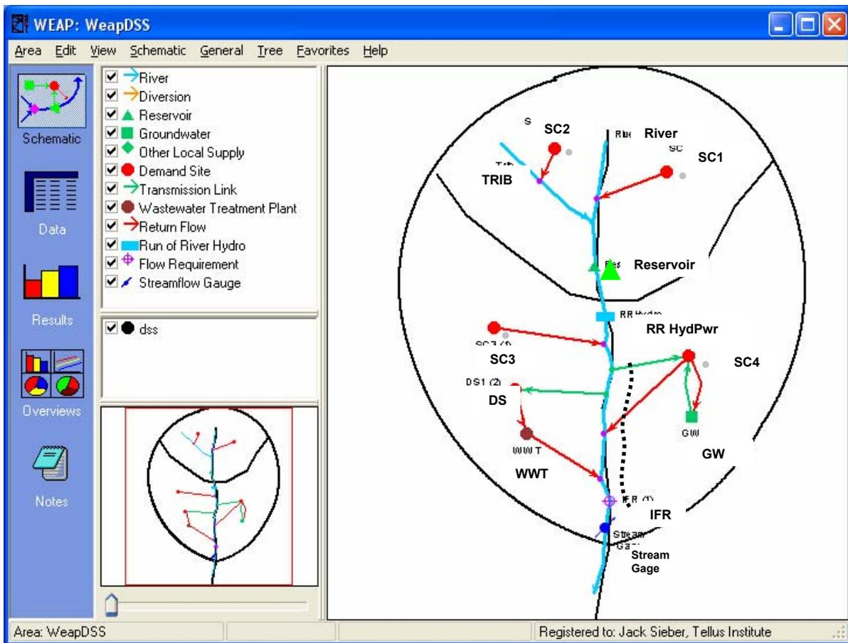
**Figure 4.2. An example of a simple watershed, sub-divided into four catchments (SC's) using the WEAP21 graphical user interface model building tools. The dark, dashed line segment on the lower portion of the river indicates the river length that is hydraulically connected to the local groundwater aquifer, GW. DS is a conventional demand site, WWT is a wastewater treatment plant, IFR is an instream flow requirement, RR HydPwr is a run-of-the-river hydropower object.**
