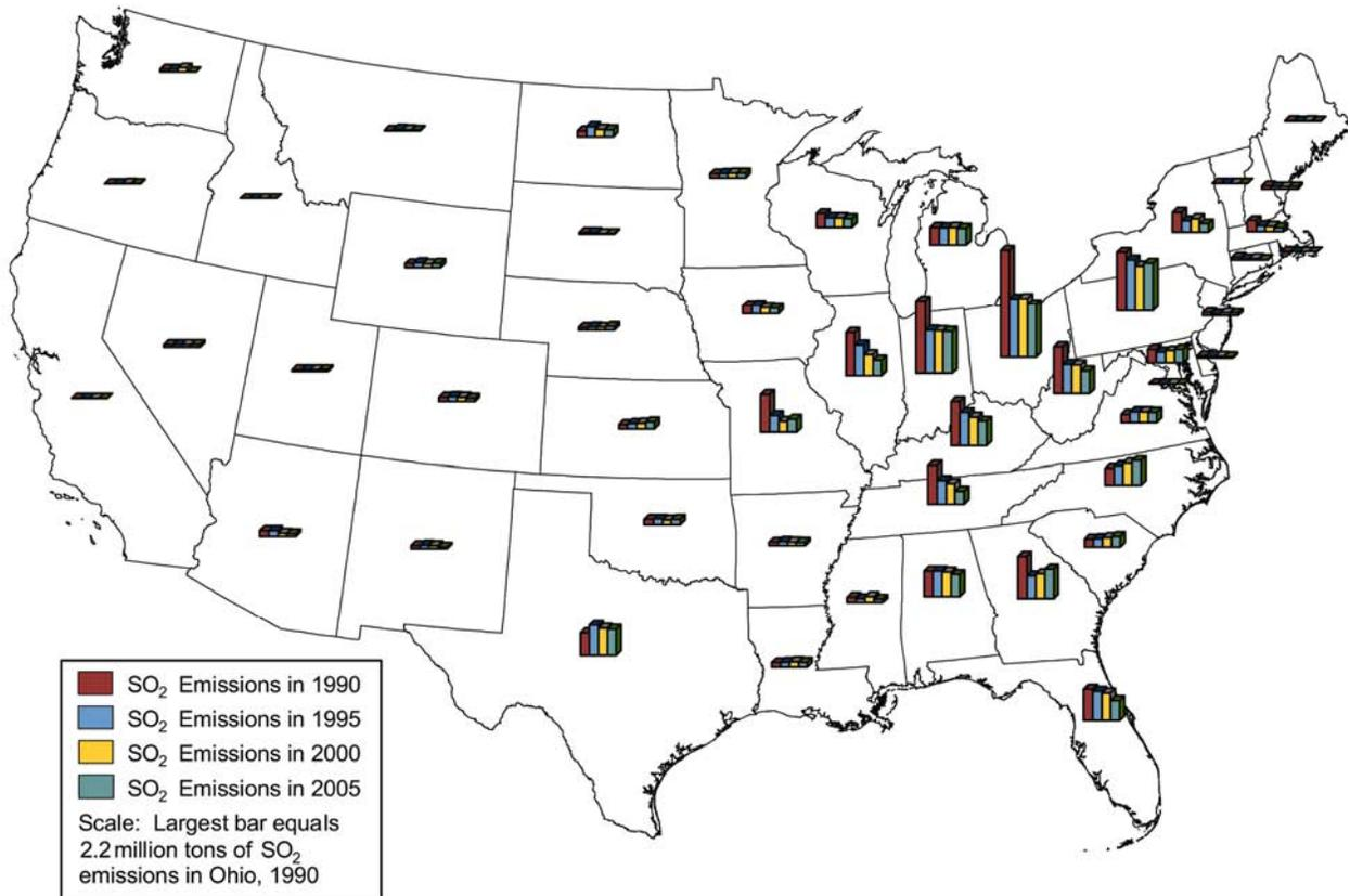
**Figure 2.4-1. State-level SO<sub>2</sub> emissions, 1990-2005.**
