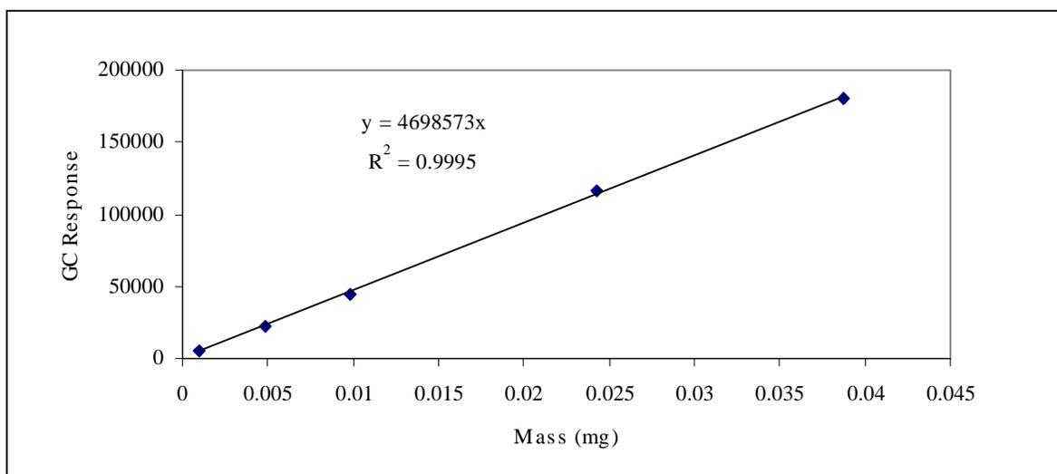
**Figure 3-5. Gas-phase calibration curve for acetone.**
