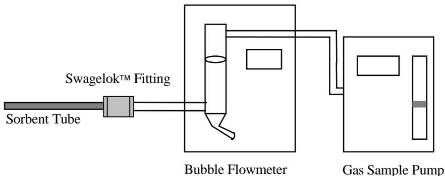
**Figure 3-1. Gas sampling experimental setup.**
