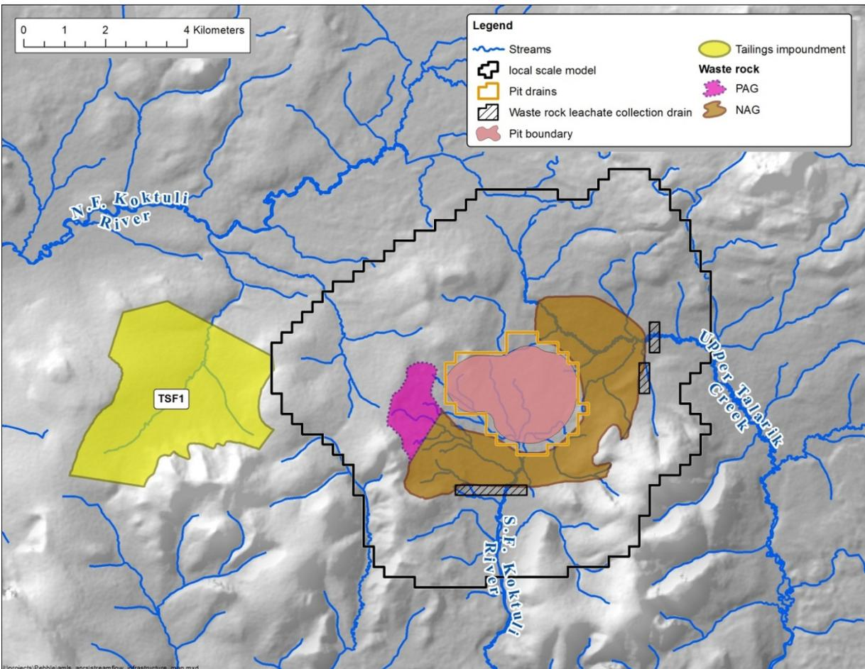
**Figure 4. Mine infrastructure used for 25-year mine scenario.** Open pit contours, waste rock geometry, and tailings impoundment digitized from Ghaffari et al. (2011). Overlays show model grids designated as drains, and spatial extent of local-scale model.
