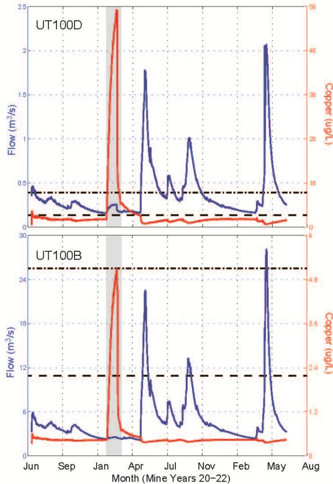
**Figure 12. Estimated copper concentrations and stream discharge in years 20 to 22: results of a one-month mitigation failure in SFK (SK100G and SK100C) and UT (UT100D and UT100B).** Dashed and dash-dot lines represent minimum and maximum values of acute hardness-based water quality criteria calculated using baseline water chemistry for each site. Vertical grey shading shows the duration of the leachate collection system failure.
