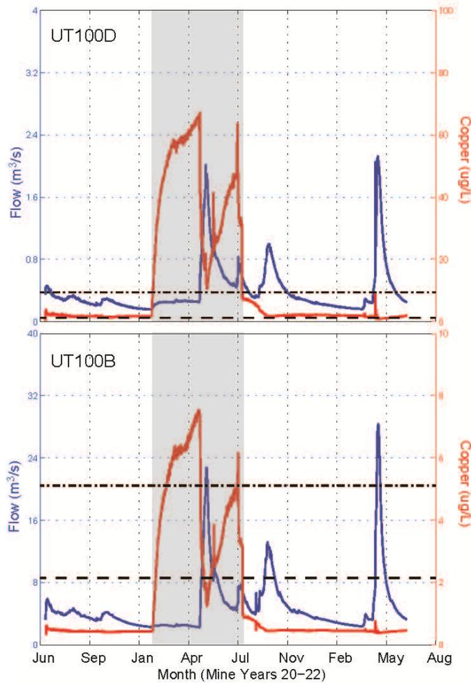
**Figure 13. Estimated copper concentrations and stream discharge in years 20 to 22: results of a six-month mitigation failure in SFK (SK100G and SK100C) and UT (UT100D and UT100B).** Dashed and dash-dot lines represent minimum and maximum values of acute hardness-based water quality criteria calculated using baseline water chemistry for each site. Vertical grey shading shows the duration of the leachate collection system failure.
