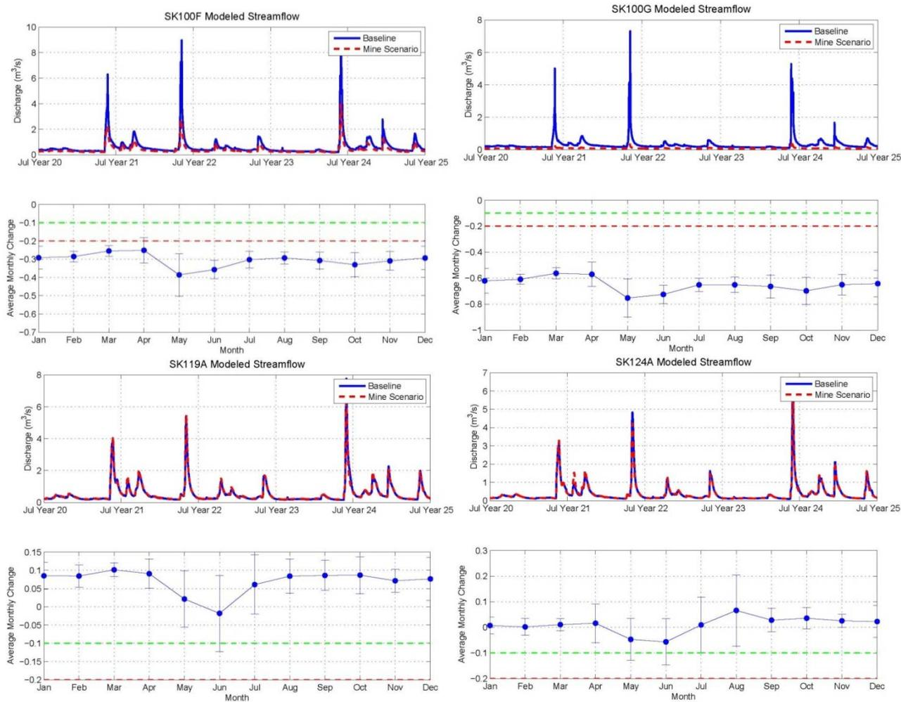
**Figure A.20. Modeled flow reductions from a large mine scenario for SFK gage stations (cont.).** In all figures, the upper plot shows the baseline and mine impacted hydrographs, while the lower plot shows the average flow change by month over the last 5 years of the model run (+/- 1 SD). Green and red dashed lines in the lower plots illustrate 10% and 20% flow reductions, respectively, for reference.
