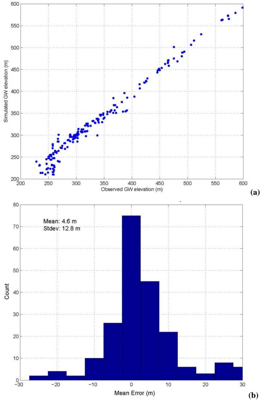
**Figure 7. Groundwater calibration results.** (a) Comparison of annual averages of observed and simulated groundwater elevations throughout the model, and (b) histogram of mean errors in groundwater depths from all locations.
