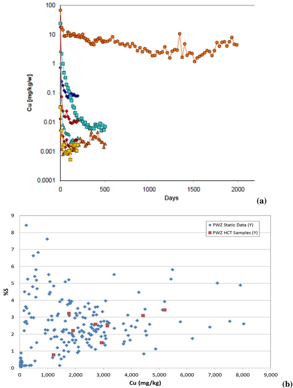
**Figure 5. HCT samples.** (a) Copper release rates in plutonic Pre-Tertiary waste rock samples (SRK Consulting, 2011b, Appendix 11G); [w = week; all samples shown are Pre-Tertiary plutonic rocks (primarily granodiorite); trends and copper concentrations were similar for sedimentary/volcanic Pre-Tertiary rocks (primarily mudstone)], (b) Pebble West Zone (PWZ) static and HCT comparison for samples from units containing Pre-Tertiary mudstone: % sulfur and copper (SRK Consulting, 2011b).
