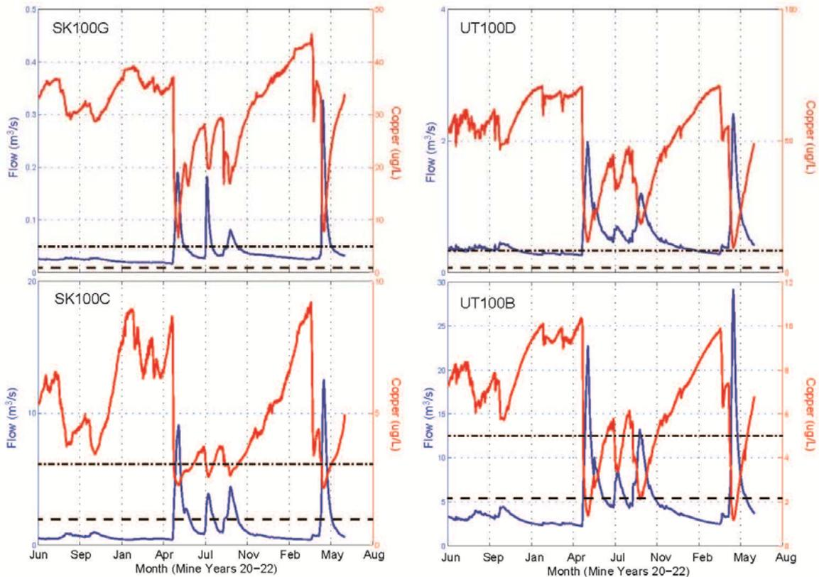
**Figure 11. Estimated copper concentrations and stream discharge in years 20 to 22 with no mitigation: results in SFK (SK100G and SK100C) and UT (UT100D and UT100B).** Dashed and dash-dot lines represent minimum and maximum values of acute hardness-based water quality criteria calculated using baseline water chemistry for each site.
