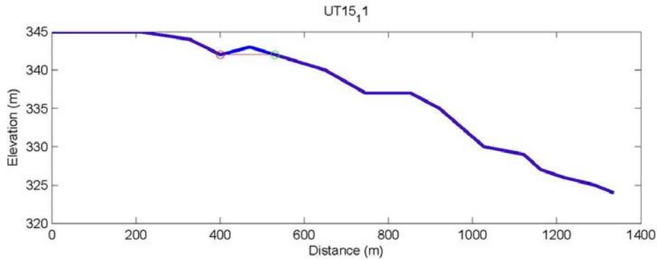
**Figure A.11. Example of spike removal process for surface streams.** Blue line is raw river elevation profile. Red line is corrected elevation profile. Note removal of spike at a distance of approximately 450 meters, between red and green circles.
