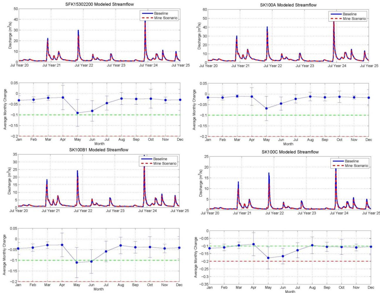
**Figure A.20. Modeled flow reductions from a large mine scenario for SFK gage stations.** In all figures, the upper plot shows the baseline and mine impacted hydrographs, while the lower plot shows the average flow change by month over the last 5 years of the model run (+/- 1 SD). Green and red dashed lines in the lower plots illustrate 10% and 20% flow reductions, respectively, for reference.
