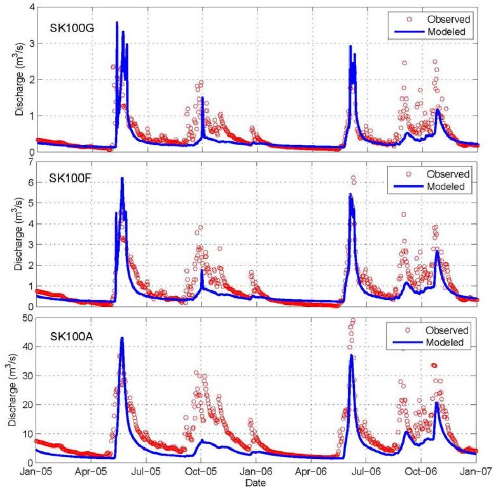
**Figure 6. Examples of calibration run results for streamflow in the upper, middle and lower SFK. Note general agreement between magnitude of spring peak and baseflow, and timing of baseflow recession.**
