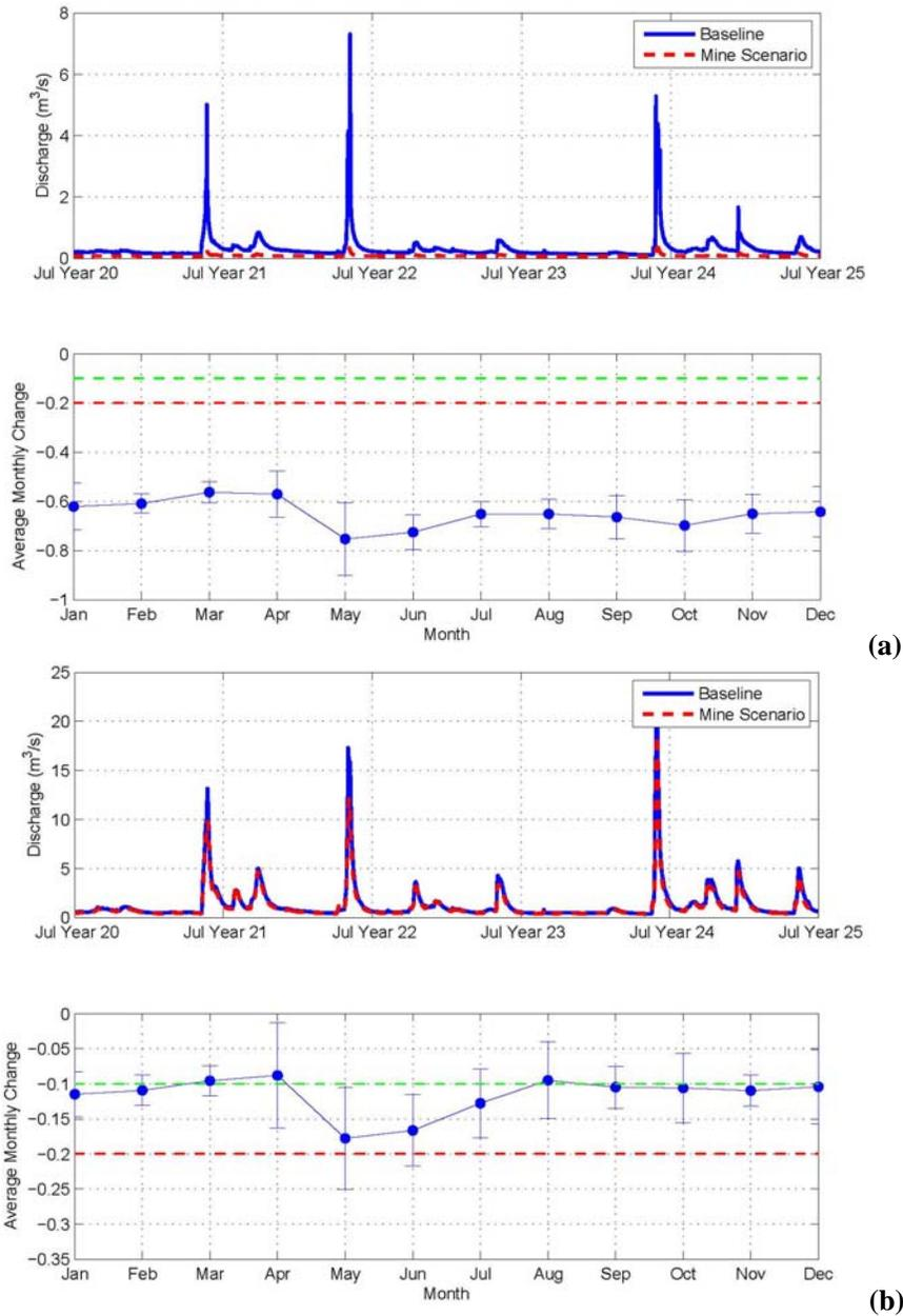
**Figure 10. Hydrographs showing modeled changes in streamflow from a 25-year mine plan for (a) upper SFK (SK100G) and (b) middle SFK (SK100C).** In each figure, upper plot shows pre- and post-mine hydrographs, and lower plot shows average monthly changes in flow (+/- 1 standard deviation) over model years 20–25. Dashed green and red lines in lower plots show 10% and 20% streamflow reductions, respectively, for reference. Streamflow changes for all gages are included in the appendix.
