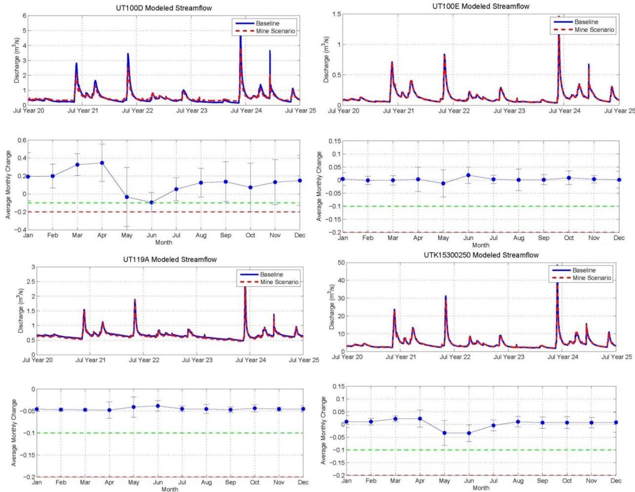
**Figure A.21. Modeled flow reductions from a large mine scenario for UT gage stations.** In all figures, the upper plot shows the baseline and mine impacted hydrographs, while the lower plot shows the average flow change by month over the last 5 years of the model run (+/- 1 SD). Green and red dashed lines in the lower plots illustrate 10% and 20% flow reductions, respectively, for reference.
