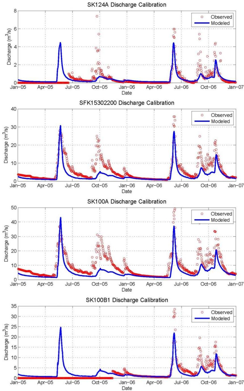
**Figure A.17. Comparison of observed and predicted streamflow at SFK gage stations for calendar years 2005 and 2006. Dates with zeros for observed flows in SK124A and SK100B1 reflect days without observational data**
