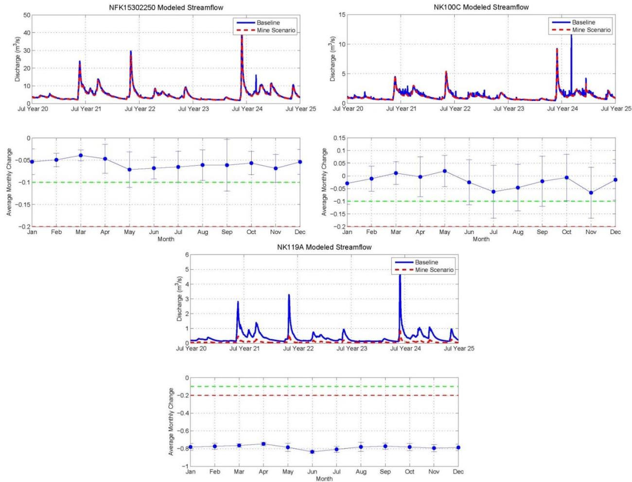
**Figure A.19. Modeled flow reductions from a large mine scenario for NFK gage stations.** In all figures, the upper plot shows the baseline and mine impacted hydrographs, while the lower plot shows the average flow change by month over the last 5 years of the model run (+/- 1 SD). Green and red dashed lines in the lower plots illustrate 10% and 20% flow reductions, respectively, for reference.
