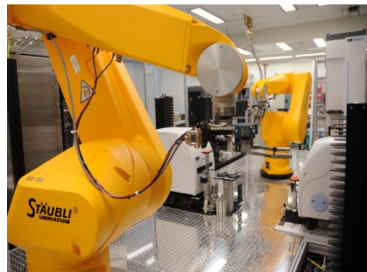
Figure 1. Toxicology in the 21st Century (Tox21) robot conducts bioassays on 10,000 chemicals. A robot arm (foreground) retrieves assay plates from incubators and places them at compound transfer stations or hands them off to another robot arm (background) that services liquid dispensers or plate readers. Photo by Maggie Bartlett (NHGRI 2012).
