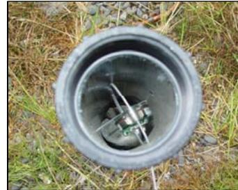
Glue the female adapters to each end of the PVC pipe. Drill a hole for one eyebolt to go through a clean out plug. Drill at least 20 holes in PVC to allow water flow. Secure the eye bolt through the clean out plug with appropriate-sized nuts and bolt. Use a cable tie through drilled holes to suspend the data logger in the housing. Additional cable ties can be used to secure rocks in the bottom of the housing to weigh it down. Screw the clean out plugs into the female adapters.
