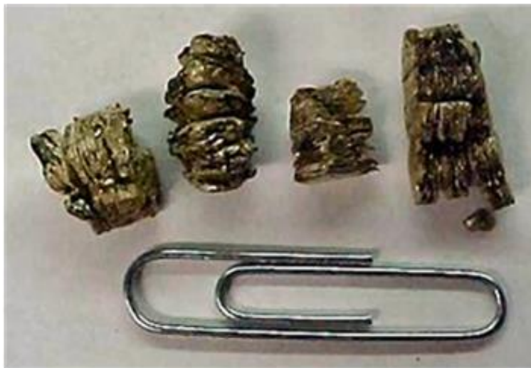
Figure 2-2. Unexpanded and expanded vermiculite.
