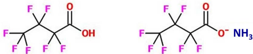
Figure 1-1. Chemical structures of perfluorobutanoic acid (PFBA) and ammonium perfluorobutanoic acid ( \text{NH}_4^+\text{PFBA} ).
