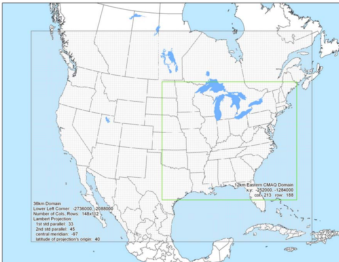
Figure 4-1. Map of the CMAQ Modeling Domain. The blue-gray outer box denotes the 36-km national modeling domain and the light green inner box is the 12-km Eastern U.S. fine grid. (Same as Figure 3-3.)
